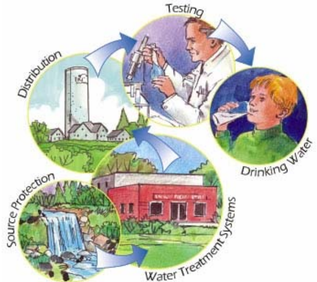
The multi-barrier approach to the provision of safe drinking water includes source protection, treatment, distribution, and testing
